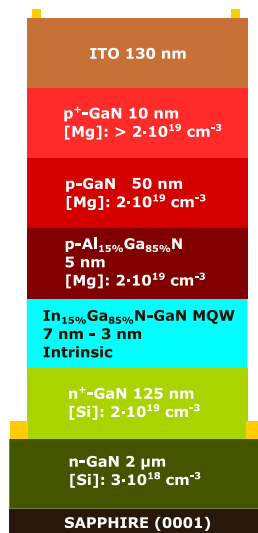
Fig. 1. ASU GaN-based solar cell with InGaN-GaN MQWs structure: the thickness and doping of each layer are presented in the figure.
